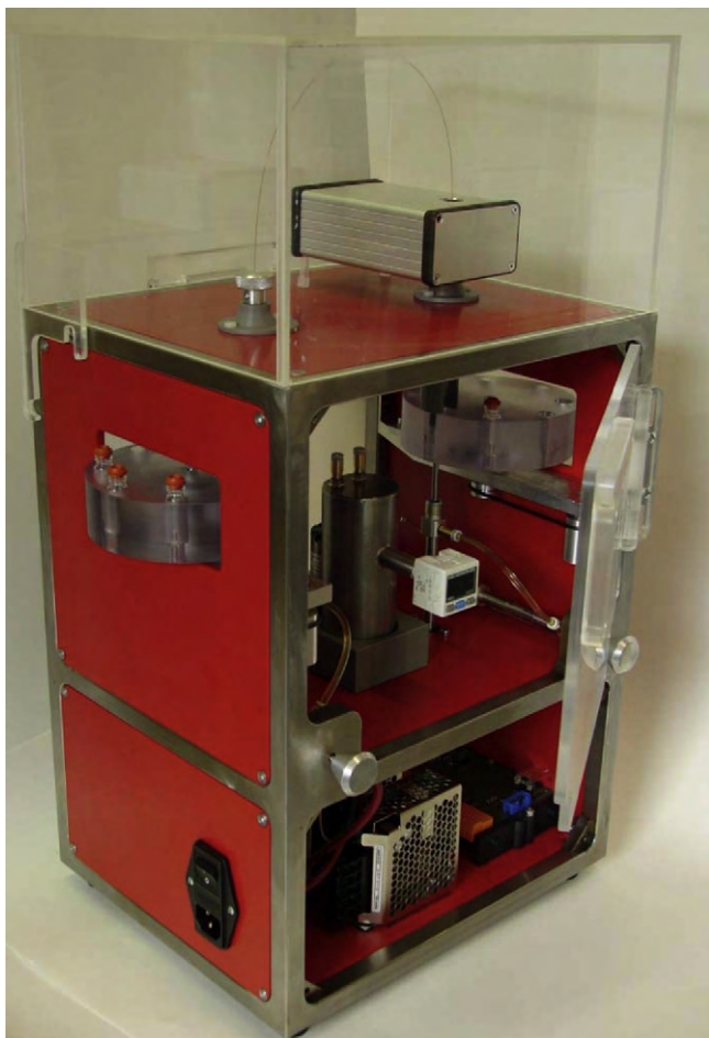
Fig. 2. Capillary electrophoresis budget device (ECB2).
